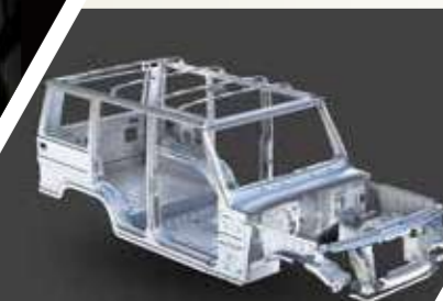
Tough & rugged body shell with a frame based construction
